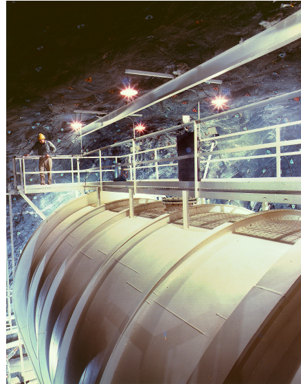
Figure 6: The Homestake mine tank: diameter - 20', length - 48', capacity - 100,000 gallons of perchloroethylene, location - 4,900' below ground surface.[12]
