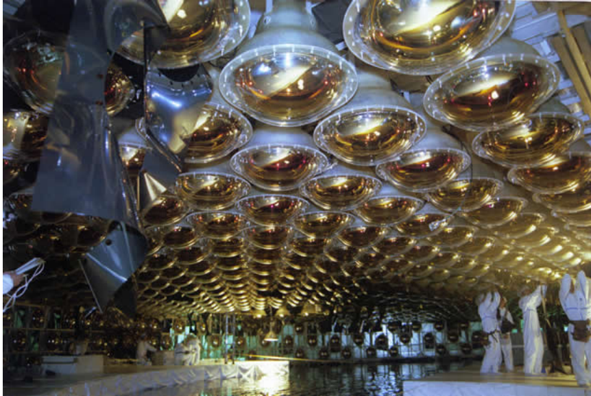
Figure 10: Array of photomultiplier tubes inside the Super-Kamiokande detector. [17]
